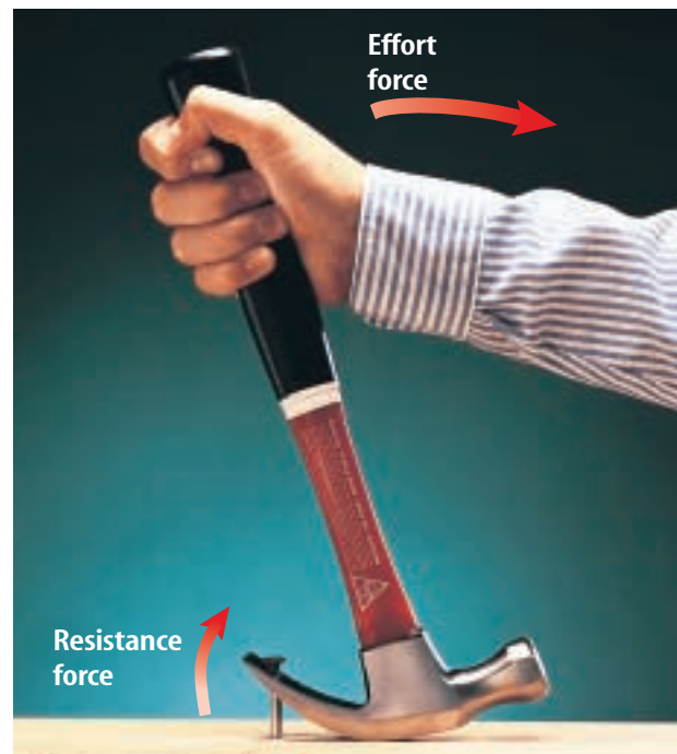
Figure 10 When prying a nail out of a piece of wood with a claw hammer, you exert the effort force on the handle of the hammer, and the claw exerts the resistance force.
